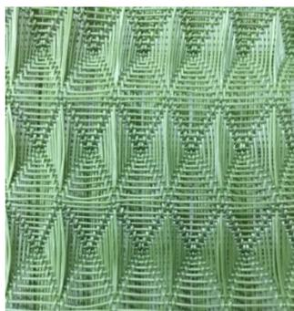
**Original Life** completes the development of Eco-friendly TRM, which features flexibility and long-term performance. It's made of PP (polypropylene) and PE (polyethylene), having three-dimensional conical structures. **Original Life** Eco-friendly TRM is woven by highly complicated method, of which the structure is uniformed. Therefore, our mat has high performance, and it is stable, durable, and function persistent.
